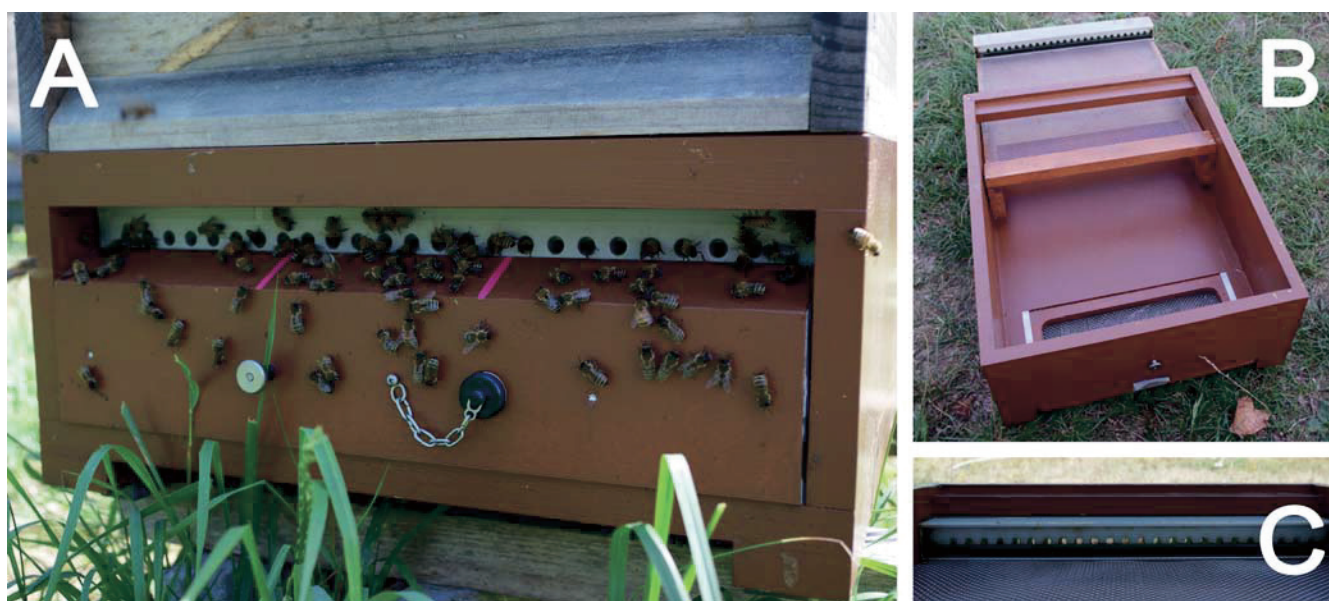
Fig. 2. BeeCheck device. A: Front view of the BeeCheck device. B: Hive bottom with the entrance tubes mounted on an exchangeable drawer tablet. C: Close-up of the 24 entrance tubes (rear-view).
